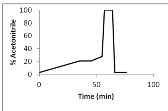
**Figure 1.** Concentration of acetonitrile during the HPLC gradient of elution
