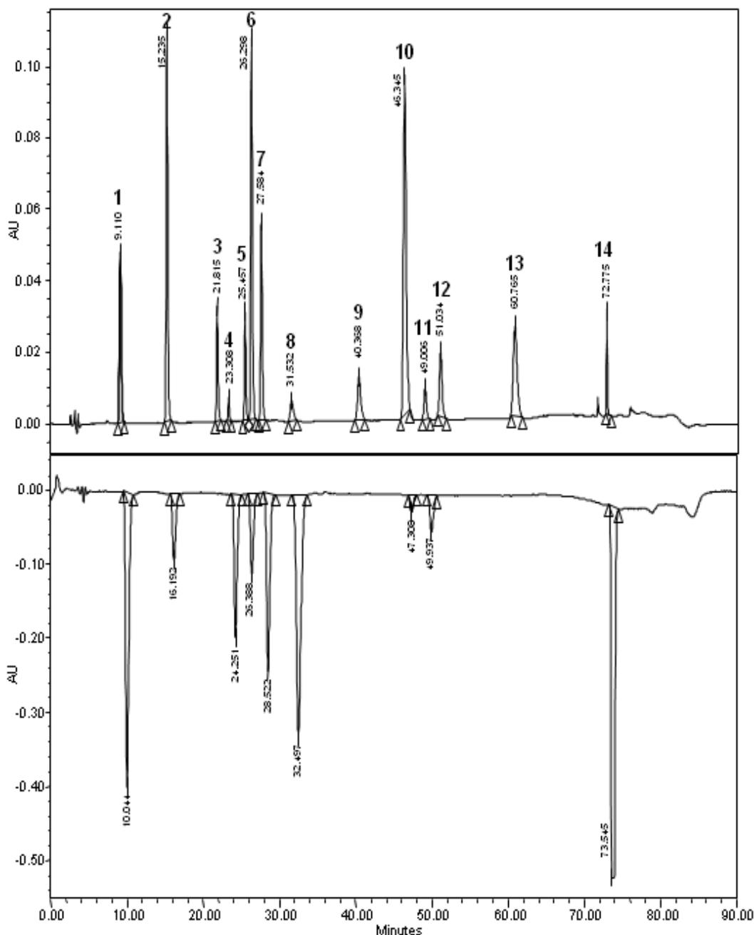
**Figure 4.** Chromatographic separation of a mixture of several polyphenols, each of the same concentration. 1:gallic acid, 2:protocatechuic acid, 3:p-hydroxybenzoic acid, 4:catechin, 5:chlorogenic acid, 6:vanillic acid, 7:caffeic acid, 8:epicatechin, 9:p-coumaric acid, 10:ferulic acid, 11:sinapic acid, 12:m-coumaric acid, 13:o-coumaric acid and 14:trolox.
